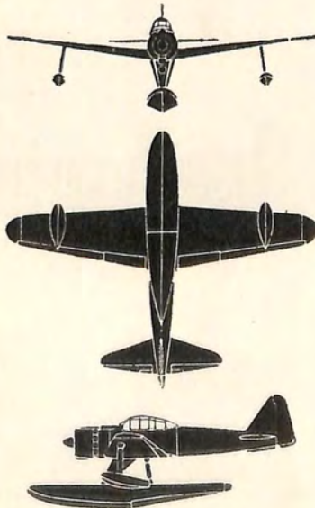
TYPE 2 FFP RUFE Span 39' 5" Length 33' 10"
